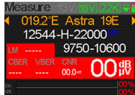
These values are highlighted in green when the signal is locked.
