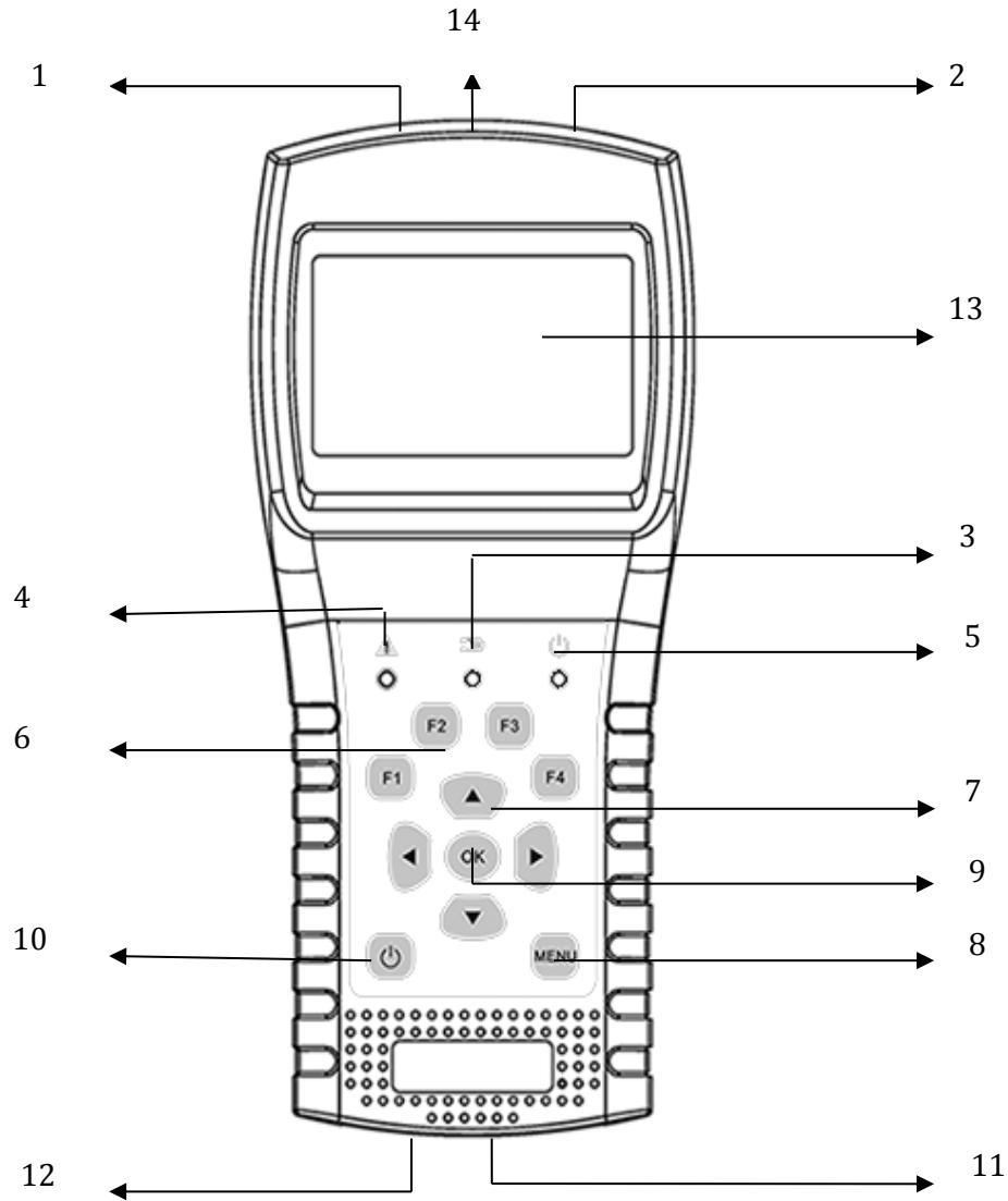
**1.RF In (Antenna Input):** input signal for standards DVB-T and DVB-C. Connect directly the coaxial cable on this outlet.
