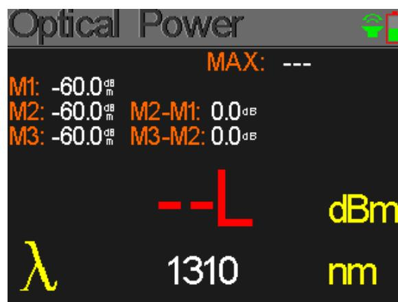
Press on [**▲ / ▼**] to change the length wave: 850, 980, 1300, 1310, 1490, 1550 and 1610 nm. Press [OK] to save the current value measured. Press on [F3] to switch the measurement mode Optical power in dBm measurement mode attenuation in dB and vice versa.
