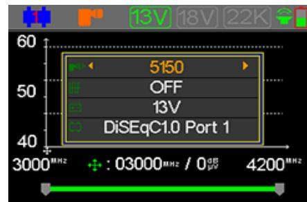
Press [OK] to check if the frethis current can be locked or not. A dialogue box appear if the transponder is locked.
